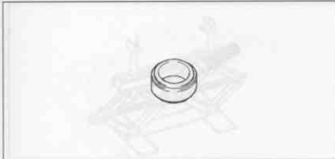
Head Pipe Outer Race Press Shaft : 57001-1075
